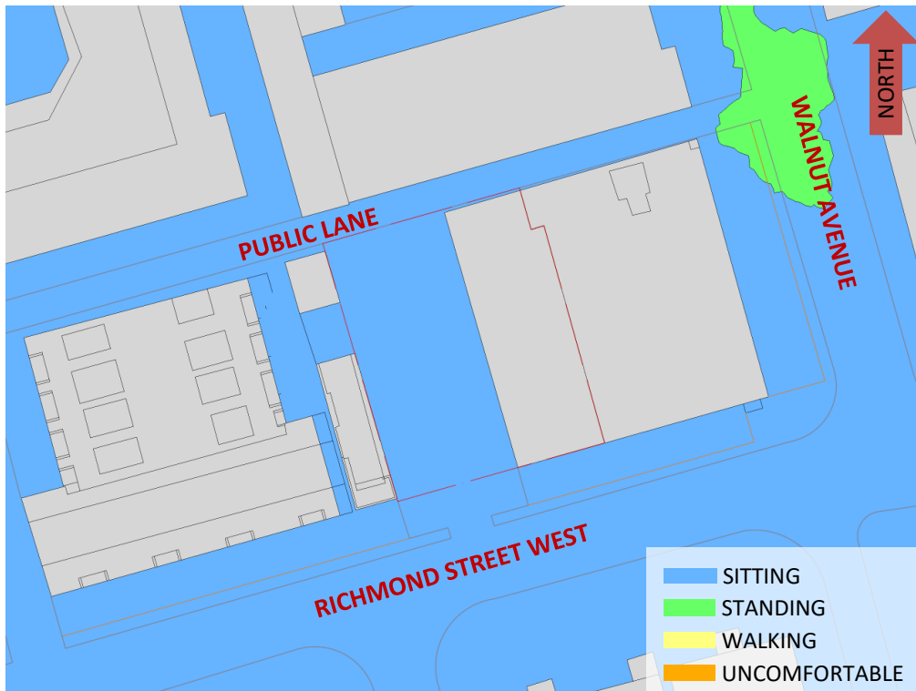
FIGURE 3B: SPRING – EXISTING – WIND COMFORT, GRADE LEVEL
