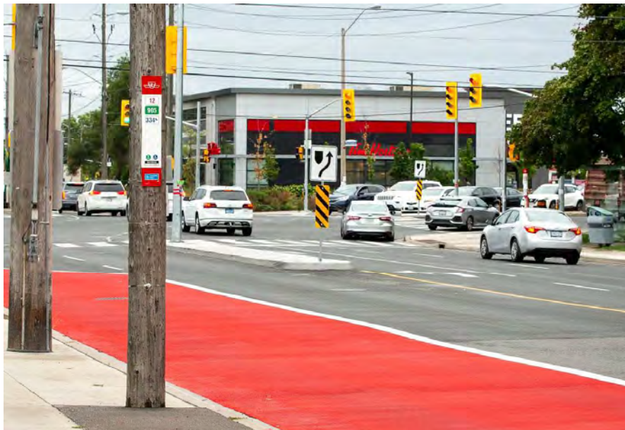
Figure 16: RapidTO Bus Lane on Eglinton Avenue East (photo courtesy of City of Toronto)
